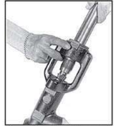
Figure 4.5: Using the seat refinishing tool
