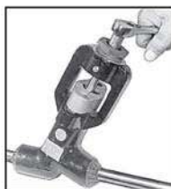
Figure 4.6: Using of socket wrench for seat-disc lapping
