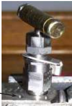
Locate the lock screw hole.
