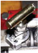
Remove Allen Screw
