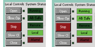
Fig 2. Indication of System Stopped (left) and System Running (right)
