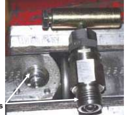
Clean and Inspect Threads
