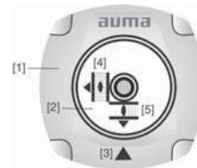
Figure 24: Mechanical position indicator
