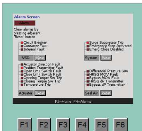
Fig 8. Trip conditions displayed on the Alarm Screen. Any fault is illuminated in red.
