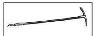
Figure 5.1A Flexible packing removal tool cork screw tip
