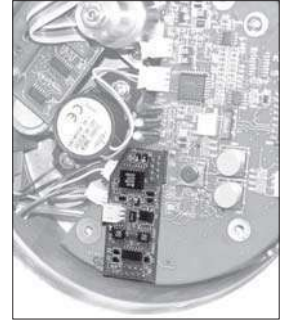
Figure 23 4-20 mA Analog Output Board
