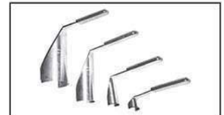
Figure 5.1B C-saw packing removal tool
