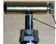
Align Flat with Hex Head Bolt
